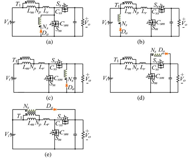
Fig. 5. ZVS synchronous boost converters with different connections of  $(p, q)$ : (a) (a, b), (b) (a, c), (c) (a, d), (d) (b, d)<sup>[23-24]</sup> and (e) (c, d).
