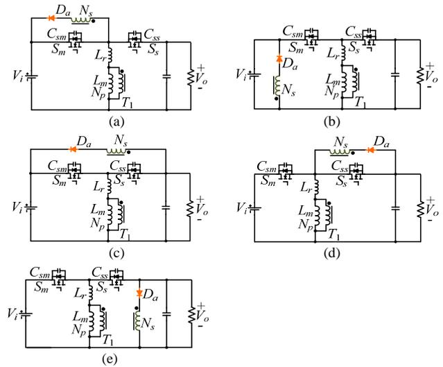
Fig. 6. ZVS synchronous buck-boost converters with different connections of  $(p, q)$ : (a) (a, b), (b) (a, c), (c) (a, d), (d) (b, d) and (e) (c, d).
