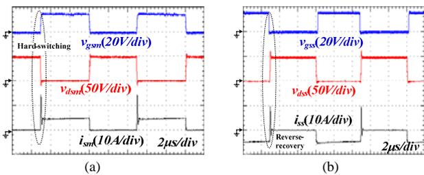
Fig. 15. Waveforms and circuit schematic of the conventional synchronous buck converter: (a) waveforms of main switch  $S_m$ , (b) waveforms of synchronous switch  $S_s$  and (c) circuit schematic.
