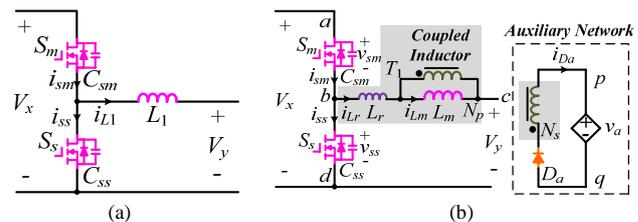
Fig. 1. Topology derivation: (a) basic cell and (b) general ZVS topology.
