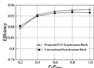
Fig. 16. Measured efficiency as a function of the output power.
