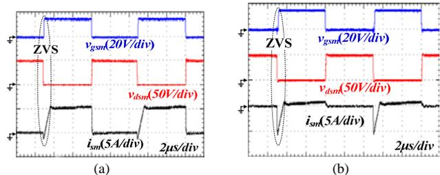
Fig. 13. Waveforms of drive signal  $v_{gsM}$ , drain-to-source voltage  $v_{dsM}$  and current  $i_{sm}$  of the proposed ZVS buck converter at different load condition: (a)  $P_{o,max}$  and (b)  $0.01 P_{o,max}$ .
