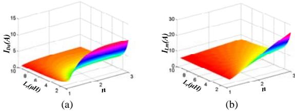
Fig. 10. Average auxiliary diode current  $I_{Da}$  and average magnetizing current  $I_{Lm}$  as a function of the leakage inductance  $L_r$  and turns ratio  $n$ : (a)  $I_{Da}$  and (b)  $I_{Lm}$ .
