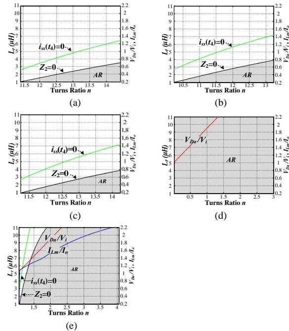
Fig. 9. Merits of ZVS synchronous buck converters at  $D=0.1$  for different connections of  $(p, q)$ : (a) (a, b), (b) (a, c), (c) (a, d), (d) (b, d) and (e) (c, d).
