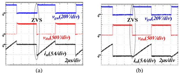
Fig. 14. Waveforms of drive signal  $v_{gsS}$ , drain-to-source voltage  $v_{dsS}$  and current  $i_{ss}$  of the proposed ZVS buck converter at different load condition: (a)  $P_{o,max}$  and (b)  $0.01 P_{o,max}$ .
