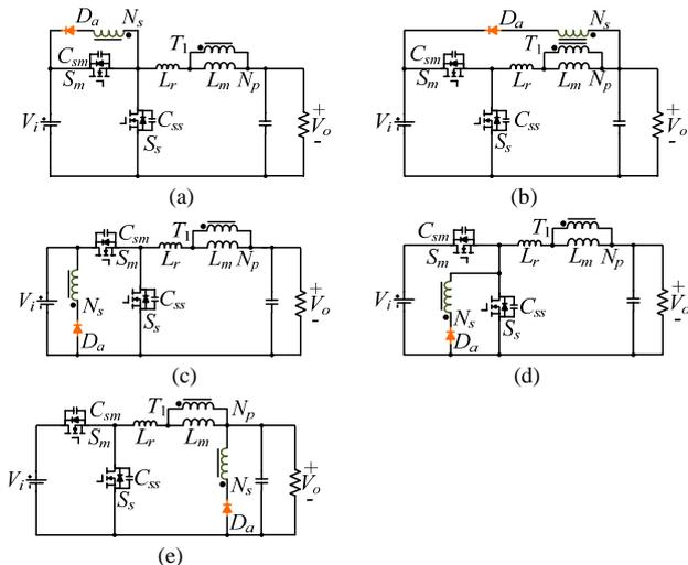
Fig. 4. ZVS synchronous buck converters with different connections of  $(p, q)$ : (a) (a, b), (b) (a, c), (c) (a, d), (d) (b, d)<sup>[5]</sup> and (e) (c, d).
