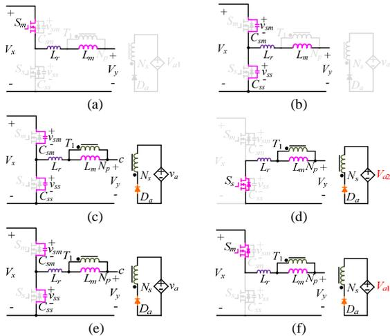
Fig. 3. Equivalent circuits of the general ZVS topology in different stages: (a) stage 1, (b) stage 2, (c) stage 3, (d) stage 4, (e) stage 5 and (f) stage 6.
