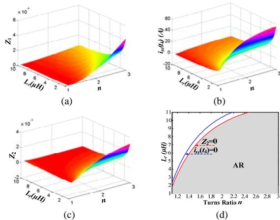
Fig. 11. The relationship of  $Z_1$ ,  $i_{ss}(t_4)$ ,  $Z_2$  and available region with the leakage inductance  $L_r$  as well as the turns ratio  $n$ : (a)  $Z_1$ , (b)  $i_{ss}(t_4)$ , (c)  $Z_2$  and (d) available region.
