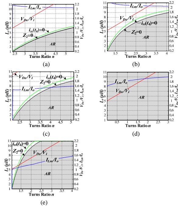
Fig. 8. Merits of ZVS synchronous buck converters at  $D=0.5$  for different connections of  $(p, q)$ : (a) (a, b), (b) (a, c), (c) (a, d), (d) (b, d) and (e) (c, d).
