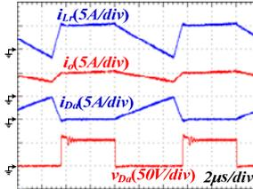
Fig. 12. Waveforms of leakage inductor current  $i_{Lr}$ , output current  $i_o$ , auxiliary diode current  $i_{Da}$  and voltage  $v_{Da}$  of the proposed ZVS buck converter at full load condition.
