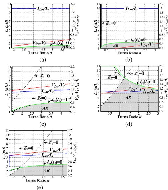
Fig. 7. Merits of ZVS synchronous buck converters at  $D=0.9$  for different connections of  $(p, q)$ : (a) (a, b), (b) (a, c), (c) (a, d), (d) (b, d) and (e) (c, d).
