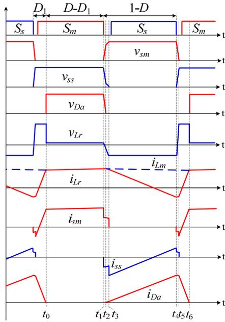
Fig. 2. Key operating waveforms.
